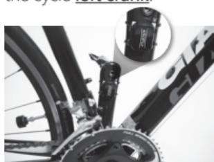
Attach the cadence sensor to the inner side of the cycle left crank for best performance
