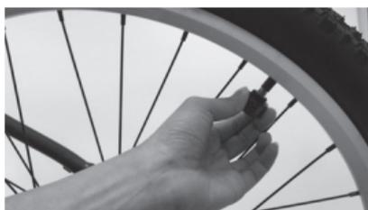
If it is a Schrader valve, AROFLY can be installed directly onto the rear valve (no need for any adaptor).
