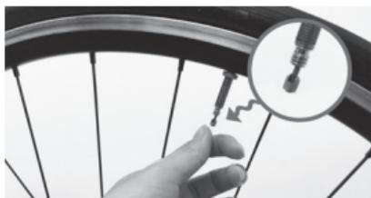
If it is a Presta valve, please loosen "the valve pin" to the top-end of the Presta valve shaft.
