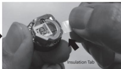
Pull and remove Insulation Tab from AROFLY to connect battery. Replace the cap to AROFLY.
